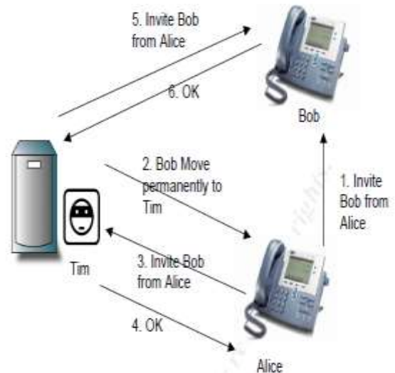
Figure 9: Illustration of Man-in-middle attack using spoof response
